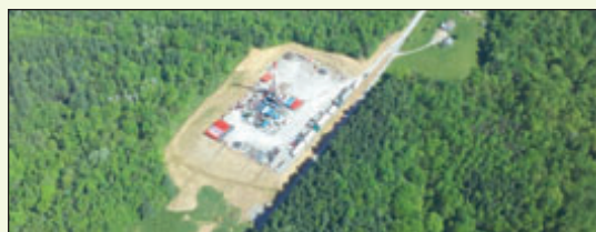
Cadastral data is in heavy demand throughout Appalachian Ohio. From coal to natural gas, 5-acre "pad sites" are created from which to fracture the Utica Shale under Appalachian Ohio.
